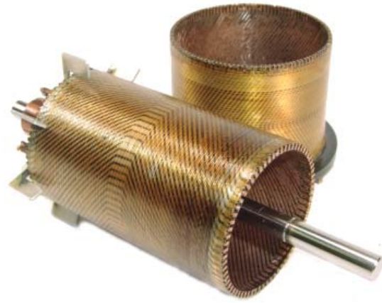
Traditional wire windings, iron or ironless-core laminations are eliminated with ThinGap's self-supporting and precision-machined copper sheet. A slotless brushless BLDC motor with a ThinGap electromotive coil demonstrates up to 92% efficiency.
