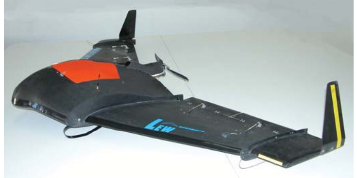
The Inventus is a state-of-the-art reconnaissance system packaged in a highly efficient, highly stable flying wing constructed from composite materials. Able to fly manually or autonomously, the Inventus E offers a line-of-sight real-time video and flight line.
