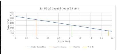
Example of Typical Use Speed-Torque Curve
