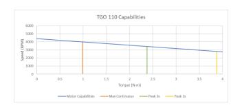
Example of Typical Use Speed-Torque Curve
