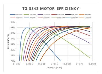
Example of Vacuum Use Efficiency Curve Torque values derated for use in vacuum. Chart assumes zero windage and uses generic bearings for the calculation. Please consult the factory if more information on assumptions used in the calculations is required.
