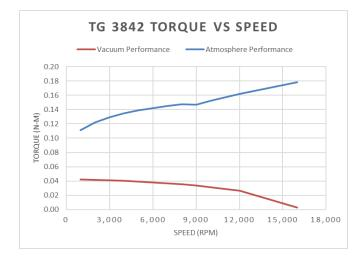
Example of Typical Use Speed-Torque Curve Higher speeds possible and is dependent on the applied voltage. Top Speed may be limited mechanically. Please consult factory if higher speeds are required
