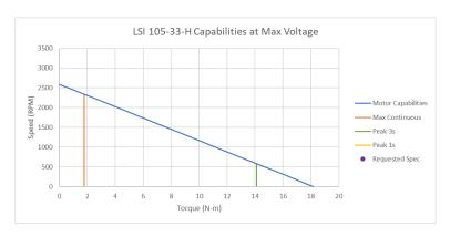
Example of Typical Use Speed-Torque Curve
